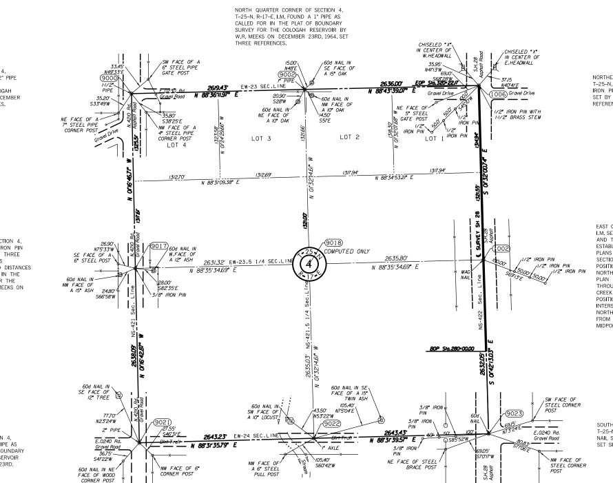
NORTHWEST CORNER OF SECTION 4, T-25-N, R-17-E, I.M. FOUND A 1-1/2" PIPE AS CALLED FOR IN THE PLAT OF BOUNDARY SURVEY FOR THE OOLOGAH RESERVOIR BY W.R. MEEKS ON DECEMBER 23RD, 1964. SET THREE REFERENCES.
